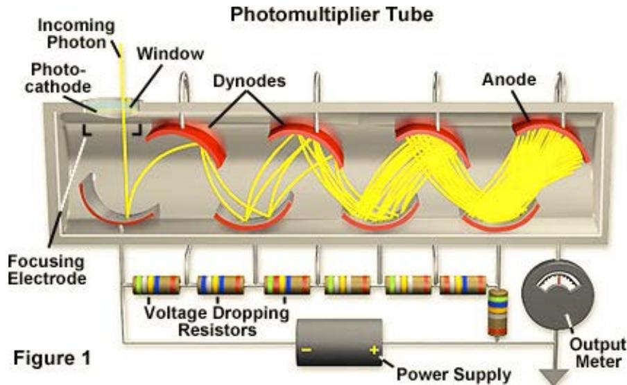
A PMT is a detector that transforms photons in electrons with a photocathode. It generates a current that will be amplified thanks to a large potential difference between the input photocathode and the output anode (more than 1000 V). The amplification is supported by intermediate electrodes (dynodes) with increasing positive potentials that liberate large amounts of electrons for each photo-electron impact.
