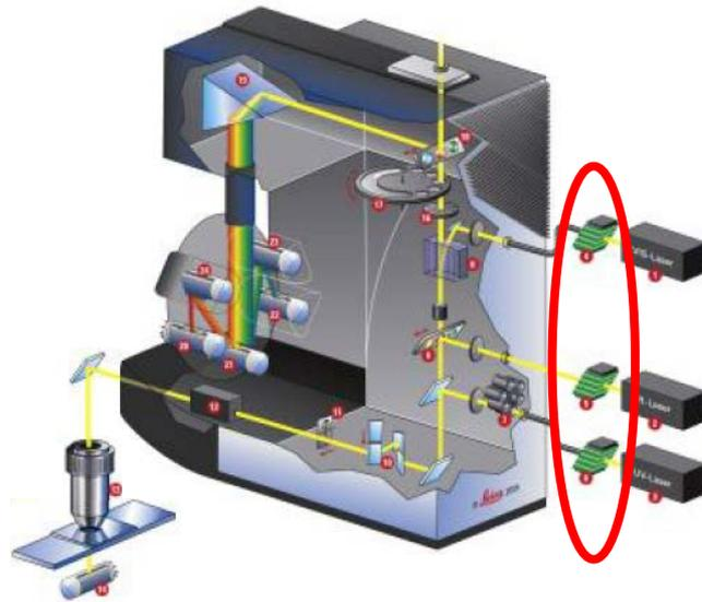
AOTF set power and wavelength of lasers in a  $\mu\text{s}$  scale time
