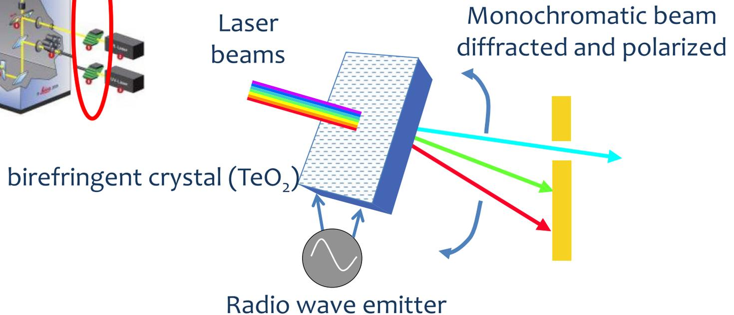
The amplitude of the perpendicular radio wave affects the transmission of the light beam and its frequency on the wavelength
