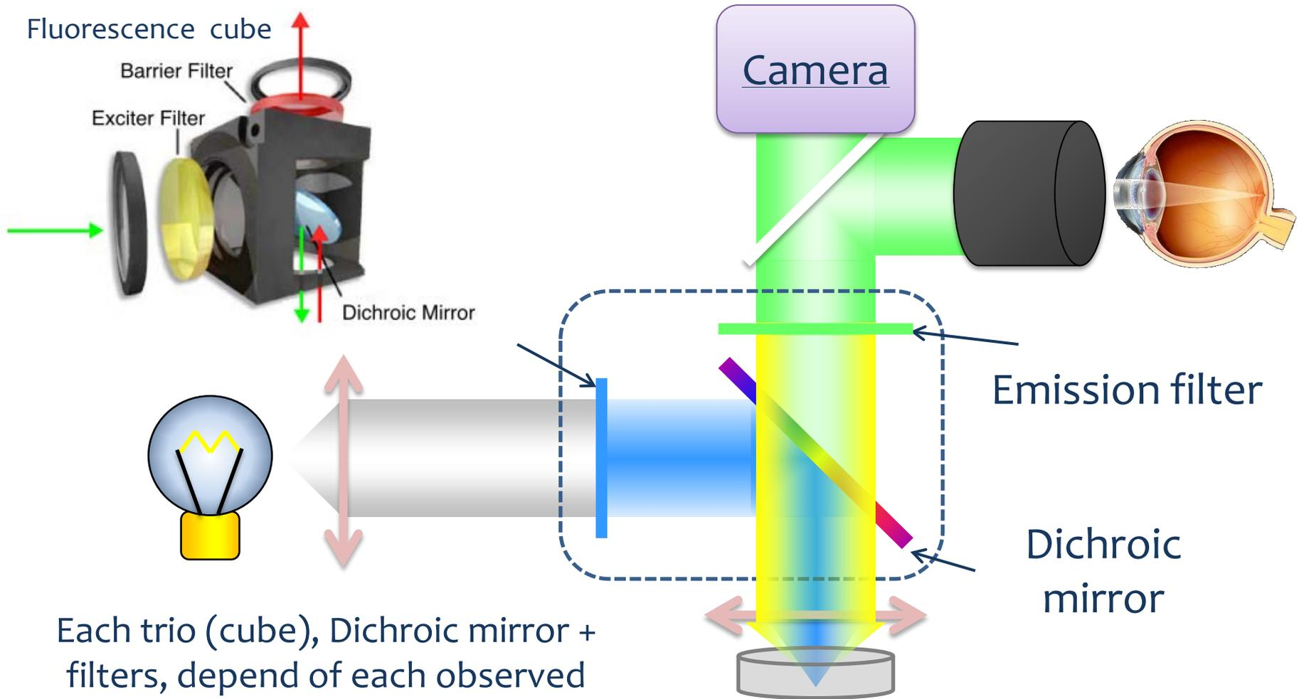
Each trio (cube), Dichroic mirror + filters, depend of each observed fluorophore individually and/or in multi-labeling
