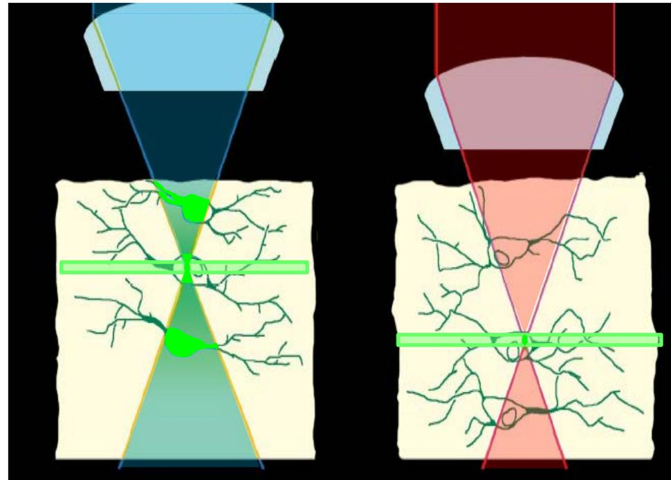
The scanning induce an optical slice intrinsically confocal, we do not need to remove out-of-focus photons (not generated).
