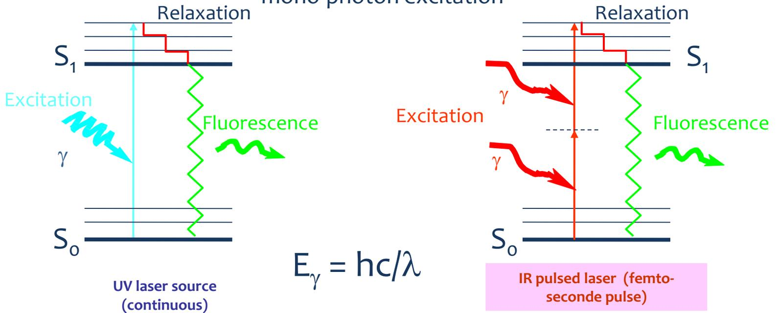
Photons have to arrive in a time window of about  $10^{-18}$  seconds (**atto**-second). This time scale is compatible with the time duration of the lifetime of this virtual state ( $10^{-17}$  seconds or 0.01 **femto**-second). They have to interact equally with the electronic cloud in a space of about  $10^{-12}$  cm<sup>3</sup>. The two-photon excitation probability is **10<sup>-30</sup>** time lower than one-photon !! (theorized by Maria Goppert-Mayer 1931 (Physics Nobel prize 1963))
