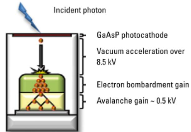
HyD's quantum efficiency is superior to standard PMTs ...
