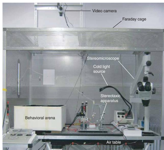
**Figure 1** | Overview of the experimental setup. Surgery as well as the processes of obtaining and anchoring a whole-cell recording are done while the animal is anesthetized and fixed in the stereotaxic apparatus. The animal is then transferred to the behavioral arena where it wakes up after it is administered antagonists to the anesthetics. While the animal performs a task, the intracellular neural signal is recorded and the behavior monitored from above with video cameras.
